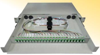
Fibre Termination Units are used for termination and management of Fibre backbone and equipment cables in Central Office and bulk fibre distribution systems. It serves as the interface between field cables and equipments. Cables may be terminated direct or after splicing. Provision has been made for internal fibre management by cable spooling with minimum bend radius and stackable splice trays. Rack mounted versions are designed for flange mounting on 19 inch racks
